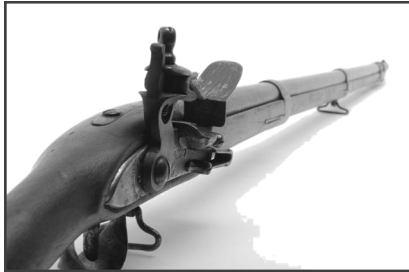
Army soldiers carried muskets like this one. With the flintlock mechanism, the soldier loaded gun powder and a lead ball separately.
